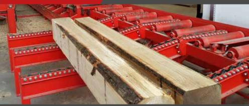
Is located infront of the band saw, where prisms move automaticaly to side transversal conveyor.
